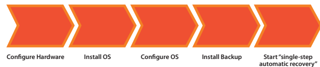
Fig 2. Physical to physical recovery process is complex and includes unreliable recovery steps that often require server rebuilds and significantly slows down recovery.
